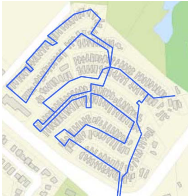
Figure 2-1 Existing Water Service Location
