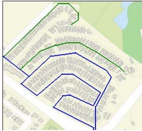
4-3-3: Piped System (blue) with Utilidor (green)
